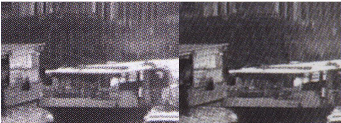
Figure 8: A 170 lpi halftone reproduced at 600 by 600 dpi/4 bits per pixel (left); a 240 lpi halftone reproduced at 1,200 by 3,600 dpi/4 bits per pixel (right)
