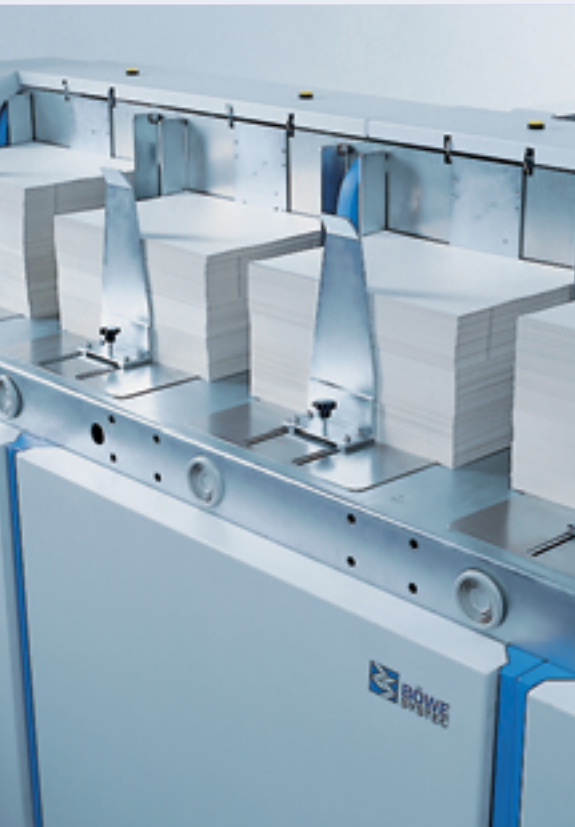
C4 enclosure feeder with high feeding capacity
