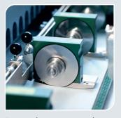
Driven edge trimmers, and up to three linear cutters
